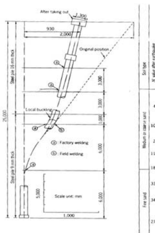
Figure 6. Pile pier no. 4, taken out from the ground after the Niigata earthquake (Fukuoka, 1966)
